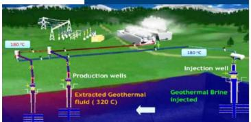
Aside from the Environmental Policy being implemented by the plant, it also established Zero Discharge System Policy wherein processed water will be re-injected to the ground through the well, where it is reheated for later
